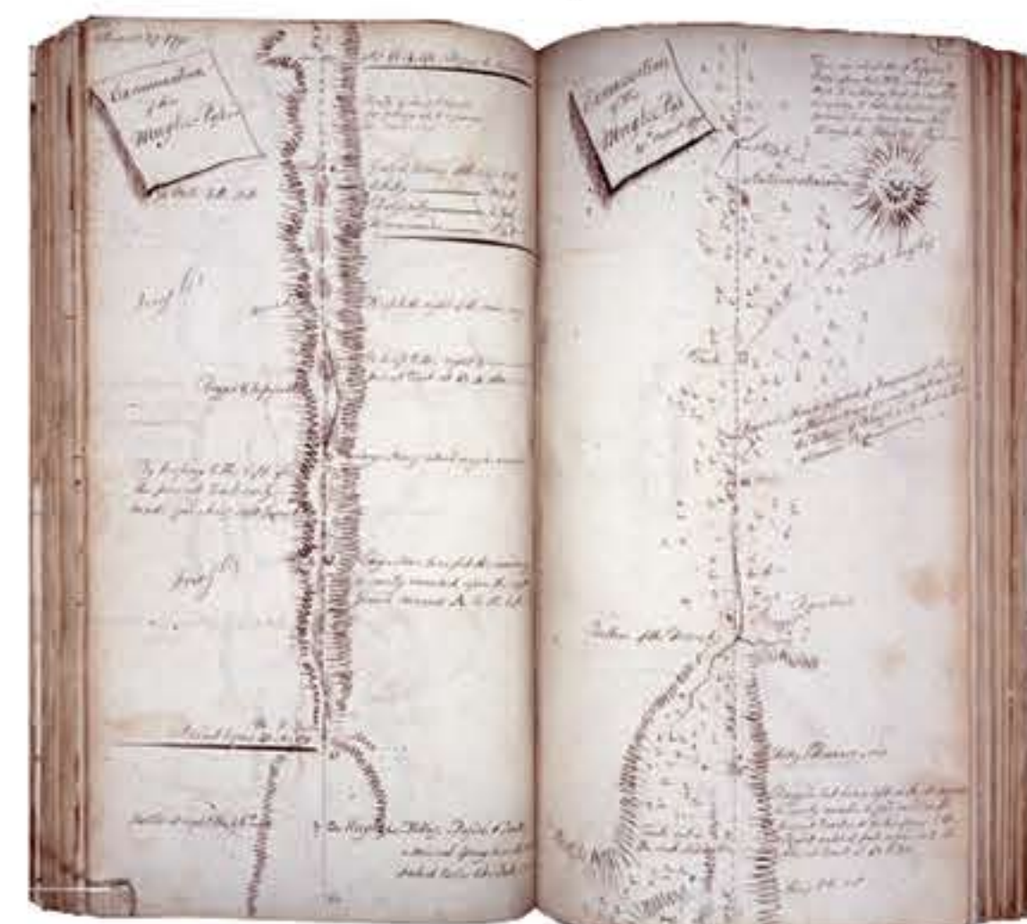
A page of Beatson's field book showing Cornwallis' army entering the 'interior' by the Moogly Pass connecting Chittoor (bottom left) and Palmaner (middle right). "This line in the middle of the page [2 inches to a mile]," writes Beatson, "represents the tract of the perambulator: upon which, are noted the distances measured; the bearings of the road by a pocket compass; the objects to the right and left, as hills, rivers, tanks or reservoirs of water, villages, forts, ravines, etc. are sketched in plan, to which are added short descriptions or remarks."
